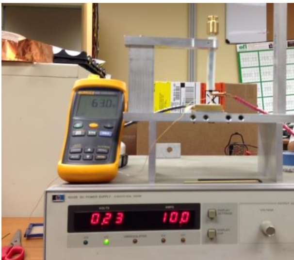
Figure 1 – Test Setup 10 amps 40 C° rise in temperature
