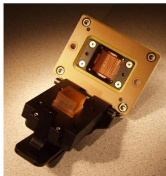
Assembled socket with an inner contactor, an outer frame and a closing mechanism
