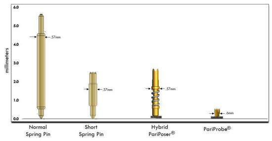
To successfully use an elastomer/PariProbe<sup>®</sup>, the DUT and the PCB needs to be flat and there needs to be a uniform load over the entire DUT. If those items are well done, high performance results will be achieved. If those items cannot be controlled, then a spring pin or a Hybrid PariPoser<sup>®</sup> will be required – even if the bandwidth results are diminished.
