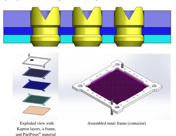
After assembly into the Kapton layers, the probes can move a bit in the Z axis. This gives the contactor some additional compliance.
