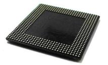
Solder ball targets of a BGA
