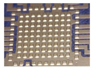
• The example below shows a further option, in case the PCB design is not accessible anymore: PariPoser material will feature punched holes under the ground plane. The material flows into the punched areas once pressure is applied. Best is to mount the material on a frame
