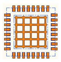
• Button plating (elevated structures) over an even ground plane.
