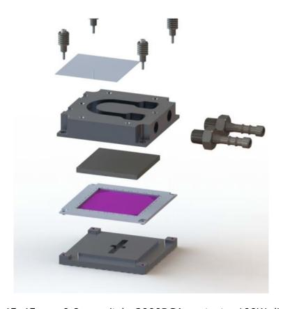
Device: FPGA 45x45mm, 0.8mm pitch, 2000BGA contacts, 100W dissipated power
