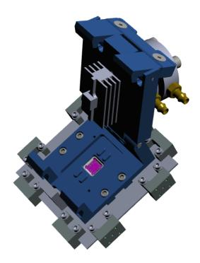
DUT: 30GHz 6x6x0.6mm BGA, 0.5mm pitch, 1300mW dissipated power
