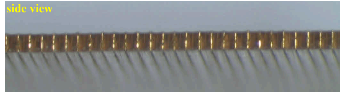
Fig.2: Photograph of an anisotropic conducting polymer with ZebraStripes™ technology to achieve conductivity in vertical direction only
