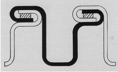
Flexible/Twistable is sealed electrically via a friction joint. This construction has the best twistable performance of all TWS waveguides. The Twistable waveguide core will hold limited pressure, but relies on the jacket for pressure sealing. Flex/Twist is not recommended for low PIM applications -use TWS seamless core.
