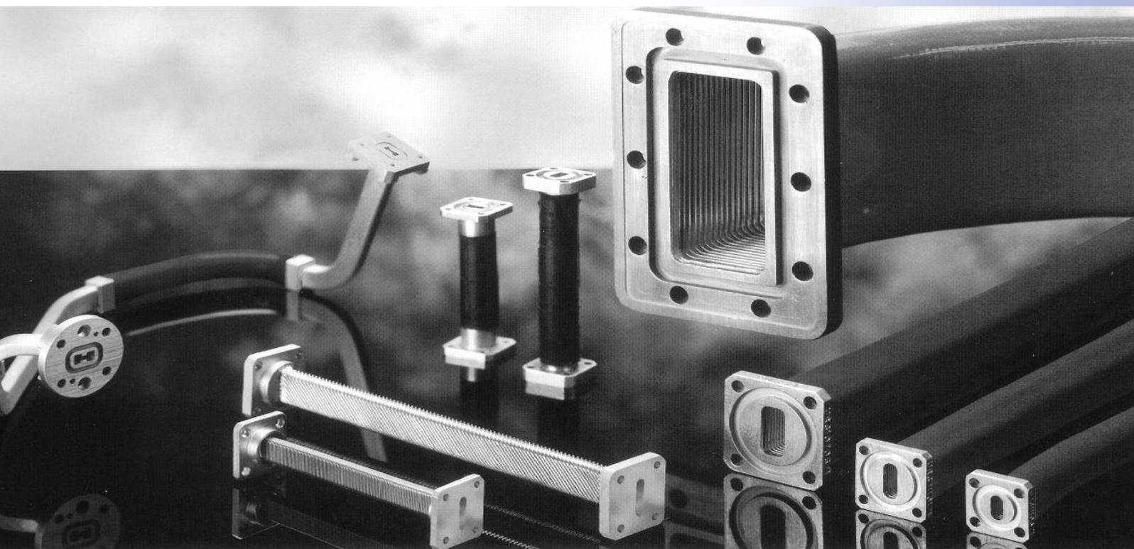
The Waveguide Solution flexible waveguides are designed to isolate vibration, eliminate installation difficulties caused by misalignment and to provide a simple aid to positioning and alignment of antennas.
