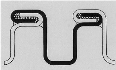
Flexible/Only core is wound with a solder fillet in the interlock, thus eliminating any RF and Pressure Leakage. Flex/Only will flex in the E and H planes only, although pre-set twists can be incorporated during manufacture.
