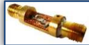
Right: Suspended Substrate Equaliser.
