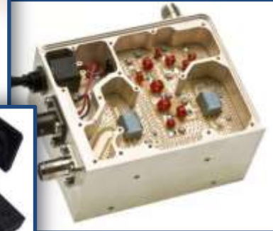
Centre: 7-Channel Lumped Element Multiplexer
