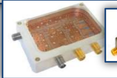
Right: Suspended Substrate Triplexer.
