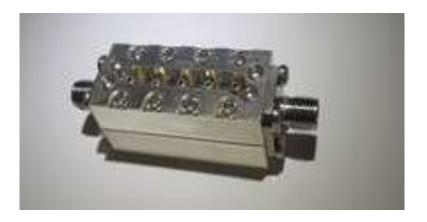
Test Piece - Dielectric resonator 26.5GHz 5<sup>th</sup>
