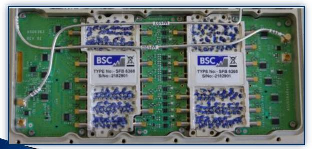
Designed for a high-spec Radio system, BSC have developed a fully-integrated 14-channel IF preselector module featuring:
