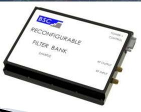
2-18GHz, 8 channel RFB Fitted to ESM suite Removes interferers on a pulse-by-pulse basis
