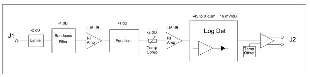
Programmable Successive Detection Log Video Amplifier (SDLVA). Used in a Fast Jet ESM platform, the SDLVA offers:
