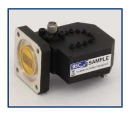
A triple-folded Ku-Band filter in WG19 (WR51) with integrated SMA transition. The space envelope 50mm x 40mm x 30mm. (2" x 1.6" x 1.2")
