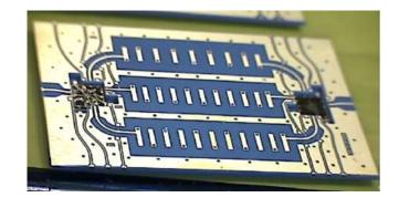
6 Channel X Band Prototype
