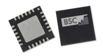
BSC are in the early stages of developing QFN -packaged tuneable Filters:-
