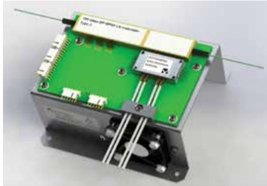
**QUAD SOA DRIVER VWA 0000905 AA for Optical Packet Switching**
