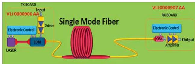
The OTX is composed by an optical laser source with a constant emitting power level at 1550nm. Then an Electro Optical Modulator (EOM) is used to convert the electrical analog signal into an optical analog signal. A driver is used to ensure the electrical dynamic required for linear operation.
