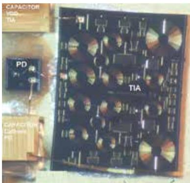
VLI 0000898 AA : S Band RF Optical receiver with TIA
